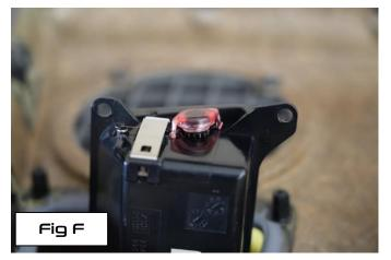
2.8. Press the rotary damper into place using moderate pressure until both tabs click into place. \*Optional for storage pocket, a dab of hot glue can be used to adhere it to the plastic trim after clicking the damper into place (Fig. G)
