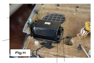
2.11. Screw in Philips fasteners until hand tight2.12. Reinstall door card back onto the door
